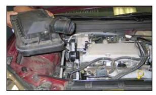
10. Remove the stock air box from the vehicle.
