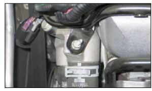
20a. On vehicles equipped with the above style heater hose tube, remove the mounting bolt shown. **NOTE: This bolt will be reused in a later step**
