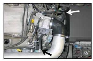
25. Cut the end of the crank case vent line, then install the provided silicone vent line onto the stock vent line and then onto the K&N® Intake Tube as shown.
