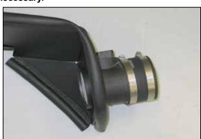
18. Install silicone hose (#08690) onto the mass air sensor with the provided hose clamp as shown.
