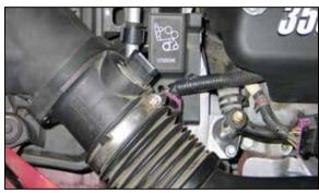
5. Loosen the hose clamp that secures the stock intake to the mass air sensor.
