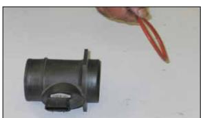
13. Remove the O-ring from the mass air sensor.
