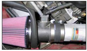
28. Re-connect the mass air sensor as shown. NOTE: Due to Manufacturer tolerances, it may be necessary to unclip the wiring harness and adjust it for more slack.
