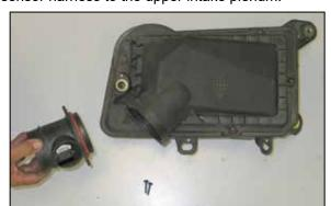
12. Remove the two Torx screws that secure the mass air sensor to the stock air box.
