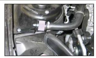
26b. Secure the air injection filter assembly to the air box mount with the provided hardware and then attach the air injection hose to the filter and secure with the provided hose clamp as shown.
