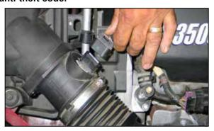
2. Depress the locking tab and disconnect the mass air sensor electrical connection.
