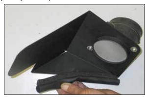
16. Install the provided edge trim (short) onto the heat shield as shown.
