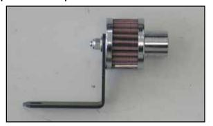
26a. On vehicles equipped with air injection system, secure the provided air injection filter to the mounting bracket (07177) as shown.
