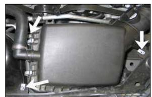
9. Remove the three bolts that secure the stock air box. On vehicles equipped with air injection, release the retaining clips and unhook the air injection hose from the air box lid.
