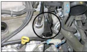
19. Install "L" bracket (#070742) to the 1/4" id hole in the engine lifting bracket using the provided hardware as shown.
