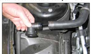
10a. On vehicles equipped with air injection, cut the clamp which secures the elbow fitting to the hose and then remove the elbow fitting from the hose.
