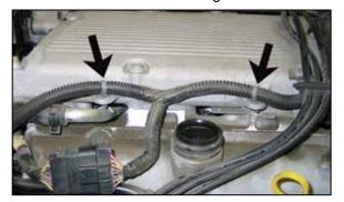
11. Remove the two clips that secure the mass air sensor harness to the upper intake plenum.
