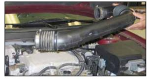
7. Remove the stock intake tube from the vehicle.
