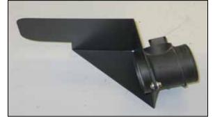
15. Install the mass air sensor onto the heat shield (07352) with the provided hardware as shown.
