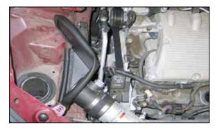
24. Install the mass air sensor and heat shield assembly. Secure with the provided hose clamp as shown.
