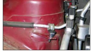
23. With the bolt removed in step #9 and spacer (#07849) secure the A/C line to the inner fender as shown.
